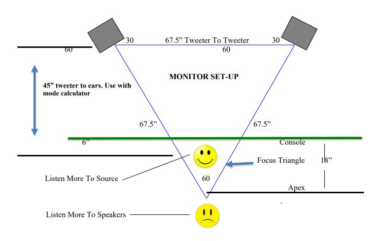
Monitor tweeter height should be at ear level, typically between 48" and 50" but could be higher or lower – measure from floor to ears.
