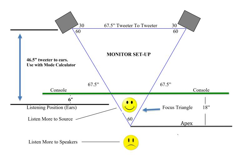
Monitor tweeter height should be at ear level, typically between 48" and 50" but could be higher or lower – measure from floor to ears.
